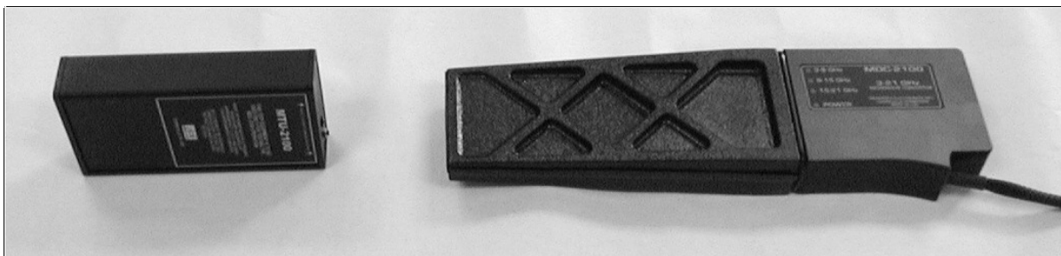
Figure 11 PROPER MTU ORIENTATION FOR TESTING BAND 2&3 (9-21GHZ) FOR MDC-2100 ONLY
